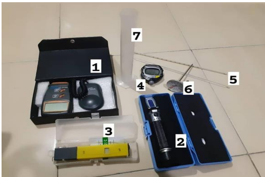
Gambar 14. (1) Luxmeter, (2) Refraktometer, (3) pH meter, (4) Stopwatch, (5) Termometer cairan raksa, (6) Termometer bimetal, dan (7) Gelas ukur 100 mL
